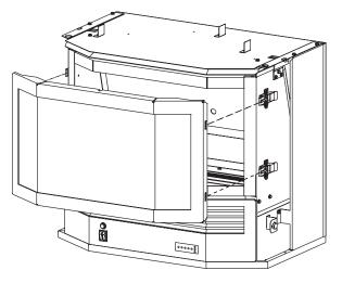
Figure 55 Front door removal drawing
